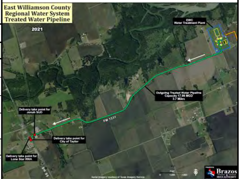
Pictured above: Proposed Treated Water Pipeline alignment
